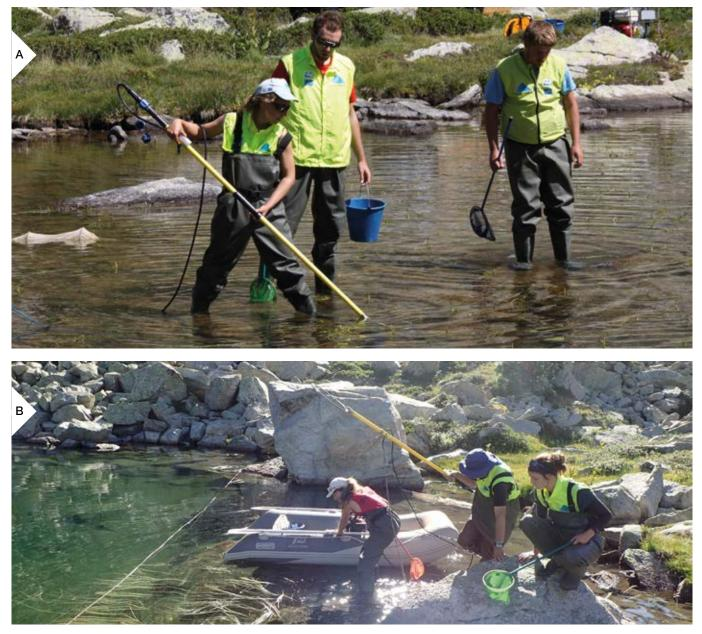
▲ Figure 4. Electrofishing in the lakes: A, use of heavy equipment; B, use of portable equipment with the operational help of a vessel and in combination with the strategic placement of shore nets.
