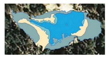
▲ **Figure 7.** Plan of the restoration of Font Grossa, where the outermost blue line indicates the perimeter of the reservoir before demolishing the dam. Blue, free water; blue-green, planting area of *C. rostrata* semi-flooded; yellow, planting area of the same species out of the water, and creation of sphagnum bogs; grey, formerly flooded area, not suitable for target mire habitats (subject to spontaneous recolonisation by meadow and opportunistic plants).
